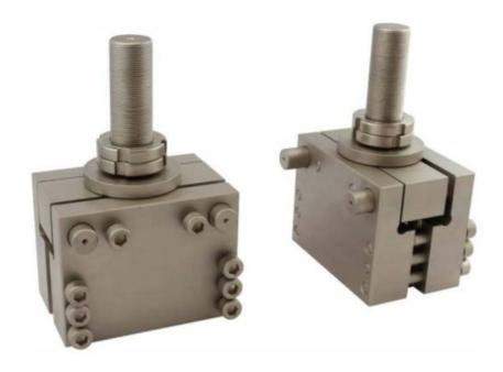
Tensile + Compression Rating: 100kN or about 22,250 lbs.
