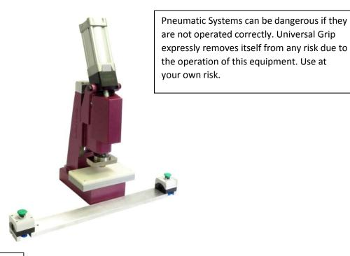
Air switch is engaged if both buttons are pressed within 0.05 seconds.
